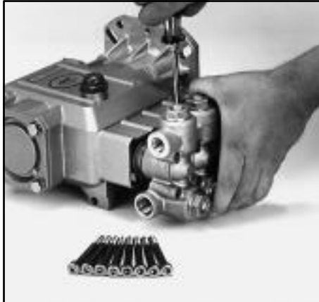
Figure 3: Removal of Seal Case and Lo-Pressure Seal
