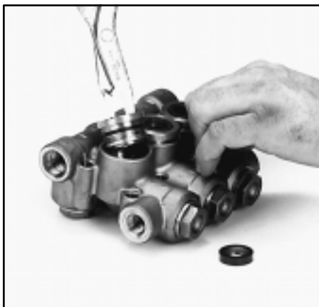
Figure 4: Removal of Seal Case and Lo-Pressure Seal
